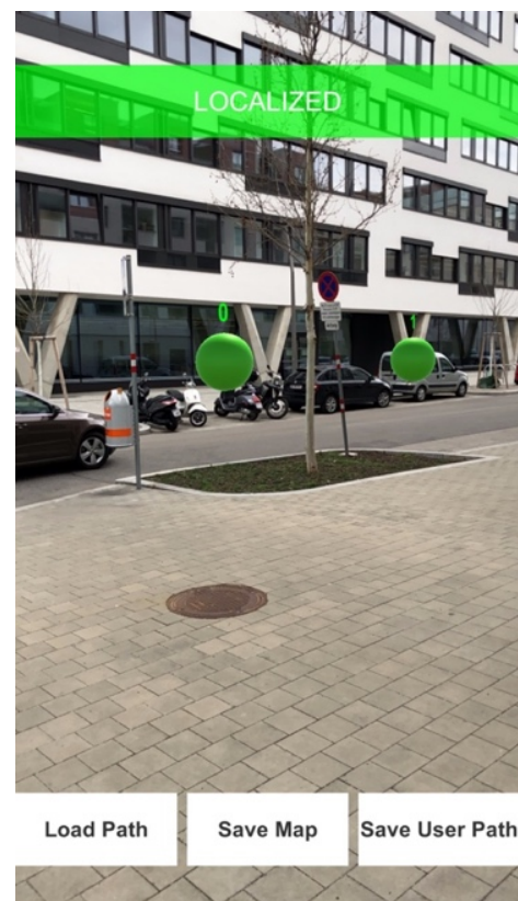
Figure 1 – Screenshot of the current prototype during use in the street. We can see two waypoints and below, buttons to load a new path and to save the current user path and the current world map.
