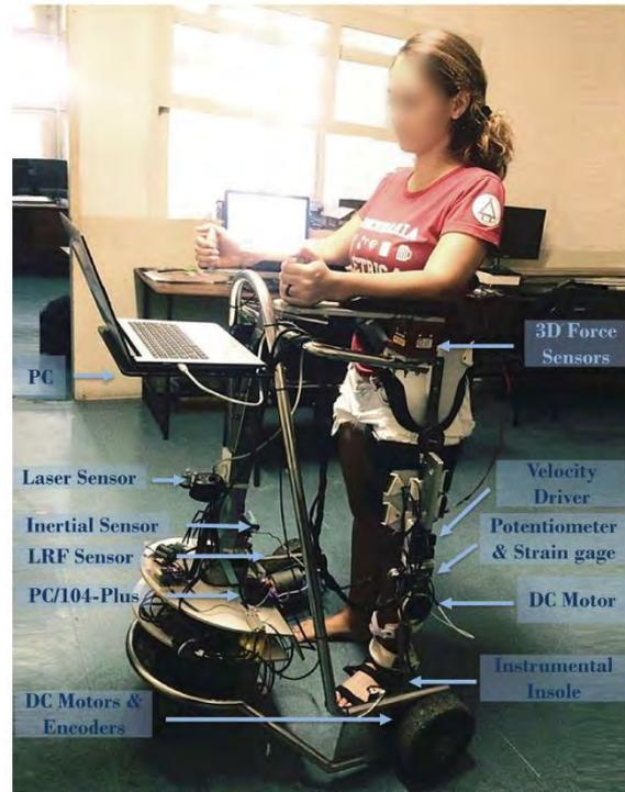
Figure 1. Robotic system for gait assistance/rehabilitation. The system is composed of exoskeleton (ALLOR) and UFES's Smart Walker (USW).
