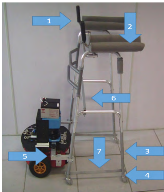
Figure 5. Robot adaptation to work as a walker.
